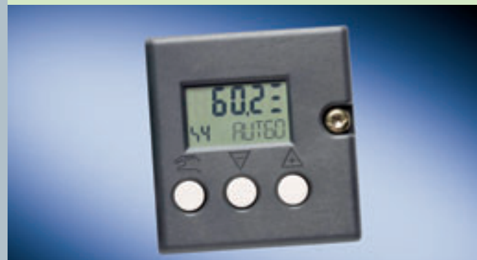
SIPART PS2 LCD: The display reports the error message (4) and the existing position (60.2) – next to it 3 bars are displayed representing the imminent positioner, valve or actuator failure (red symbol from DCS).
