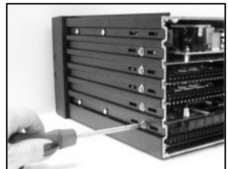
FIGURE 6.4 The Earthing Screw
