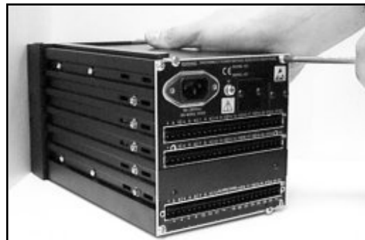
FIGURE 7.1 Removing the rear panel
