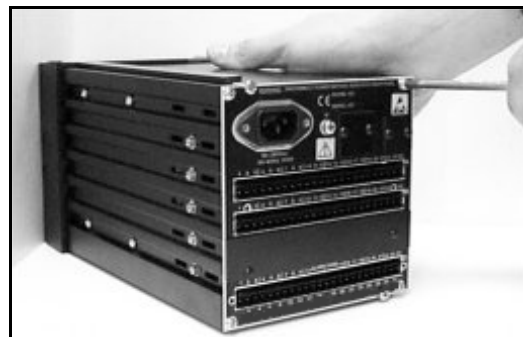
FIGURE 5.1 Removing the rear panel
