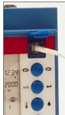
Panel mount unit with Dolphin Plus communications connection via an RJ-11 jack on the instrumentation face.
