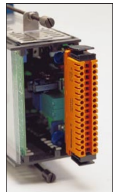
Data link to a host computer, PLC or DCS through an optional BIC II converter.
